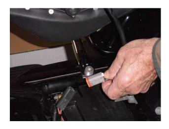
**Step 6** Check to make sure there are no folds or kinks in the wire leading from seat to receptacle before finalizing installation of seat. Engage front mounting tab first, push seat all the way forward, and insert and tighten the rear fender screw.
