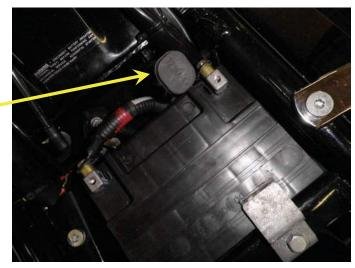
**Step 3** Remove the rubber cap from the accessory receptacle. Make sure that the receptacle is clean and free of any dirt or debris.
