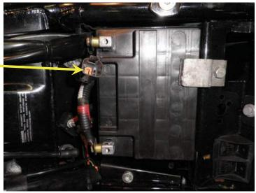
**Step 4** Prepare seat for installation. Make sure that the plug for the heating element is clean and free of any packing material. Check to see that the electrical wire is free of kinks or sharp folds. Check both switches for ease of operation; center position is off; top position is high; bottom position is low.
