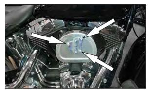
3. Remove the three air filter retaining bolts as shown.
