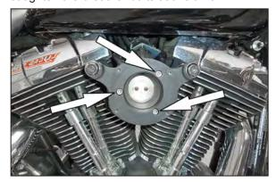
10. Install the provided gasket between the throttle body and back plate use the provided hardware to secure the back plate to the throttle housing. Tighten the crankcase breather bolts.
