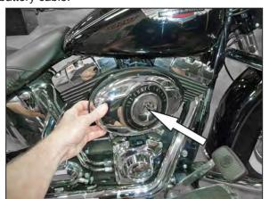
2. Remove the air filter cover retaining bolt and then remove air filter cover as shown.
