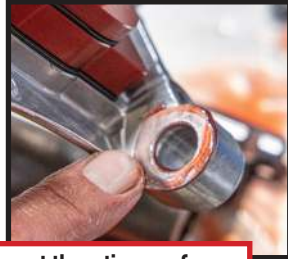
Lube rocker shafts & rocker arm support thrusting surfaces.
