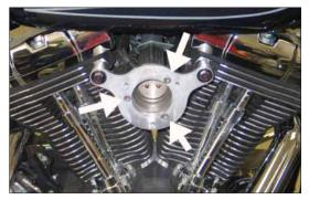
11. Install the provided gasket between the throttle body and back plate and then secure the back plate to the throttle body with the hardware provided. Tighten the crank case breather bolts.
