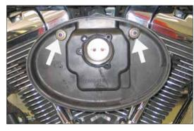
5. Remove the two crankcase breather bolts shown.
