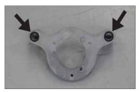
9. Install the remaining two provided o rings onto the front of the back plate as shown.
