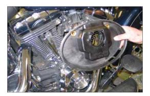
6. Remove the air filter breather base as shown. NOTE: K&N Engineering, Inc., recommends that customers do not discard factory air intake.
