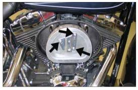
3. Remove the three air filter retaining bolts shown.
