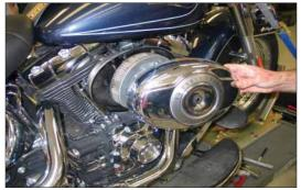
2. Remove the air filter cover retaining bolt and then remove the air filter cover as shown.
