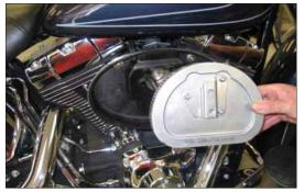
4. Remove the air filter with the breather hoses as
