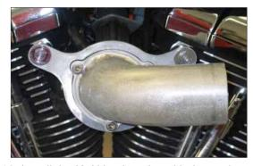
12. Install the K&N intake tube with the gasket and secure with the provided hardware.
