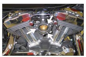
9. Install the K&N® intake tube adapter onto the throttle body using the provided hardware. NOTE: Apply one drop of the provided thread locker to the three tube adapter mounting bolts as shown.
