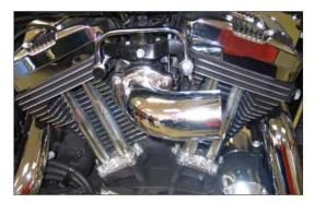
12. Install the K&N® intake tube onto the throttle body and secure with the provided hardware. NOTE: Apply one drop of the provided thread locker to the K&N® intake tube mounting bolts as shown.
