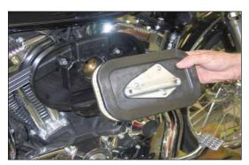
4. Remove the air filter as shown.
