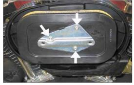
3. Remove the three air filter mounting bolts shown.
