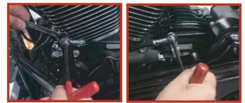
3. Compare the factory shift rod length to the RSD shift rod length. If the length is correct you are ready for installation. If the length needs to be adjusted, loosen the jam nuts using a 1/2" wrench and rotate the ball joints in or out to desired length.
