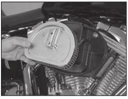
2. Remove the three bolts which secure the stock air filter element. Then remove the stock air filter element and stock crank case breather hoses as shown.
