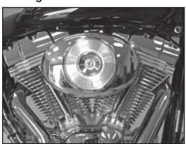
20. Reinstall the factory chrome cover and secure with the factory bolt.
