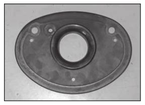
9. Install the provided velocity stack into the K&N backing plate as shown.
