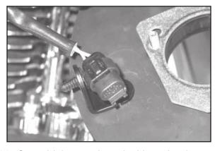
16. On vehicles equipped with an intake valve solenoid, install the intake valve solenoid connector into the bracket installed onto the rear of the backing plate. Secure with the provided tie wrap.
