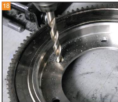
Open the holes in the ring gear with a 3/8" bit.
