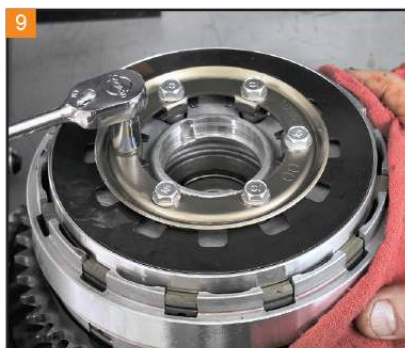
9 With a 10mm socket, remove the six bolts holding the spring retainer to the clutch hub.
