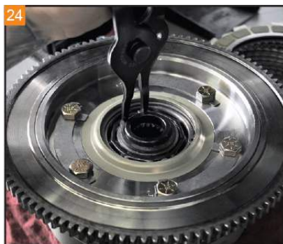
Install the retaining ring into the clutch hub from the transmission side.
