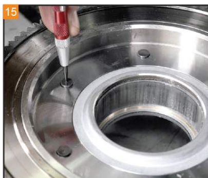
15 On the transmission side of the clutch basket, center punch the rivets holding the starter ring gear to the clutch basket.
