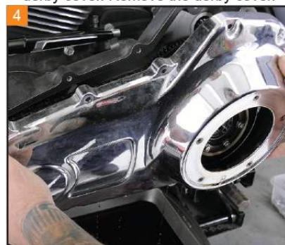
4 Remove the outer primary cover and gasket from the primary housing.
