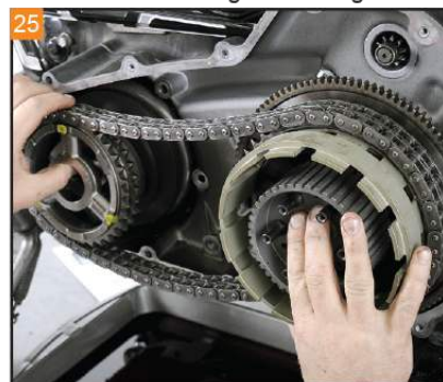
Install the clutch assembly, primary chain, and compensating sprocket. Ensure the primary chain is running the same direction as before.
