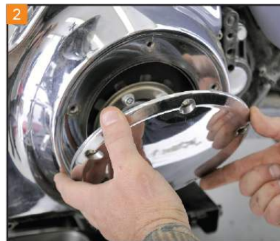
2 Remove the left side floorboard, rear left floorboard mounting bracket, heel shifter, and left passenger peg mount. Use a T27 Torx to remove the five bolts holding the derby cover. Remove the derby cover.
