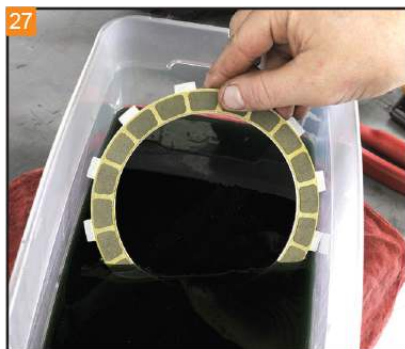
Allow the clutch plates to soak for 10 minutes prior to installation.
