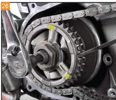
Apply red thread locker to the mainshaft nut. This nut is left hand thread. Final torque to 50-60 foot/lbs. With a new compensating sprocket bolt, torque to 100 foot/lbs., loosen a 180 degrees, and final torque to 175 foot/lbs.
