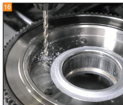
16 With a 1/4" drill bit, drill out the heads of the rivets.
