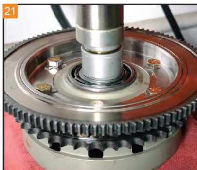
Verify the stock bearing spins freely. Press in the bearing into the Barnett Clutch Basket from the transmission side.
