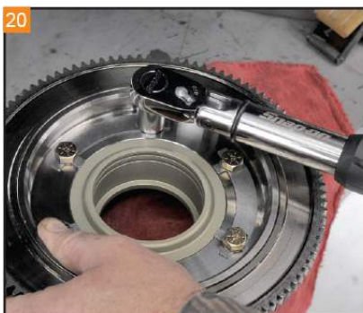
Tighten the bolts in a criss-cross pattern. Final torque of 25 foot/lbs. Bend one locking tab per bolt onto a flat of each bolt.
