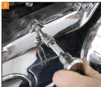
3 With a 3/16" Allen wrench, remove the bolts holding the outer primary cover to the primary housing.
