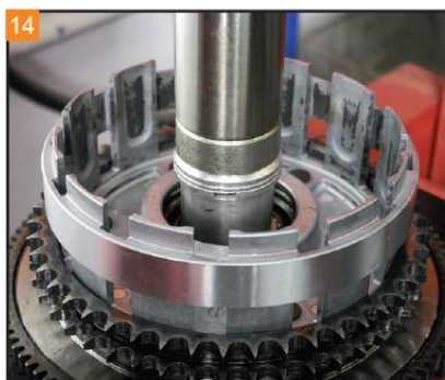
14 Position the clutch basket back in the hydraulic press. Use a driver matching the diameter of the inner race of the bearing to press the bearing out of the clutch basket.
