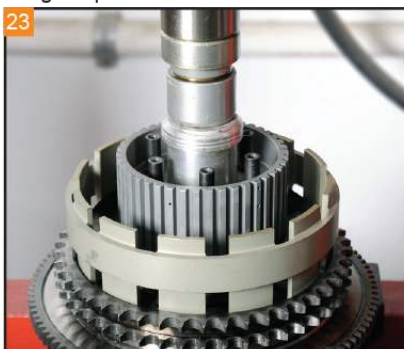
Press the Barnett Clutch Hub into the bearing.
