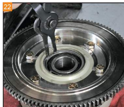
Install the retaining ring into the appropriate groove for your application, flat side facing the bearing.
