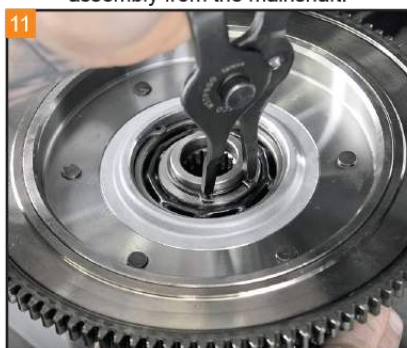
11 With the transmission side up, remove the retaining ring from the clutch hub. Wear eye protection during this step.
