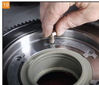
Position the ring gear over the Barnett clutch basket. Install the included bolts and locking tabs.
