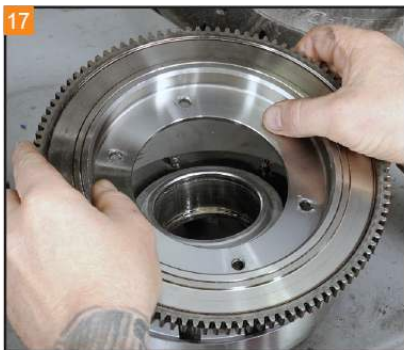
Remove the starter ring gear from the stock clutch basket.
