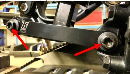
Installation of the Kodlin Lowering or Lift Kit rod:
