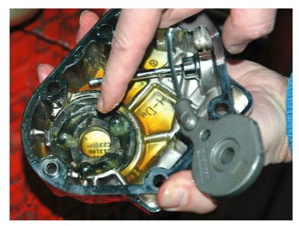
All three balls may be mounted with some grease into the Clutchlite curves. It will keep them in the correct position when the outer OEM-plate will be mounted. Watch these tree balls when mounting the OEM-plate now!
