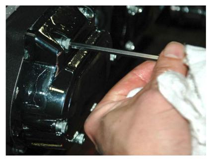
Tighten all six screws now crosswise and refill transmission oil to the correct level.
