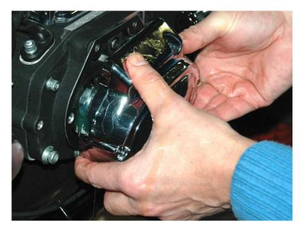
Fit clutchcable and then the cover on the transmission case but watch the two center bolts and the gasket fit.
