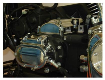
Check the transmission case cover on the right side of your bike and remove your exhaust system in case it is covering the transmission cover.
