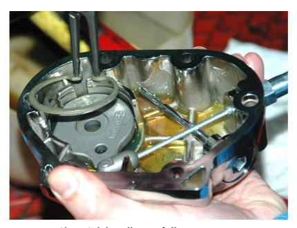
... remove the retaining clip carefully.
