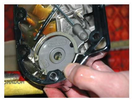
Look at the inside of the removed cover and see the OEM-clutch drive unit. The inner plate will be exchanged with the Clutchlite.
