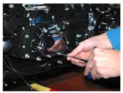
Take a clean oil bowl and put it below the transmission cover and then start removing the six screws of the transmission cover carefully with a x/x allen wrench.
