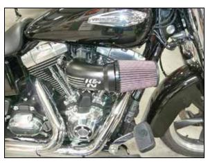
12. Install the K&N $^{\mbox{\tiny B}}$  air filter onto the intake tube and secure with the provided hose clamp.
