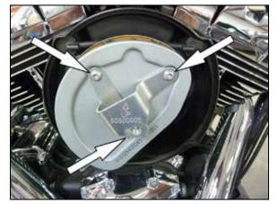
4. Loosen the three air filter retaining bolts as shown.
