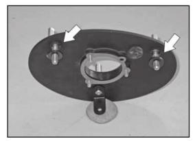
15. Install the factory breather bolts through the K&N back plate. On 2006 and later model year fuel injection models and all carbureted models, install the provided thick spacers (06403) onto the breather bolts as shown.
