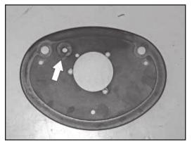
8. On vehicles equipped with a carbon canister, install the provided grommet into the backing plate as shown.
