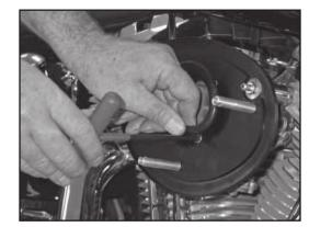
NOTE: Apply the supplied thread locker to the threads of the three supplied stand-off bolts.
