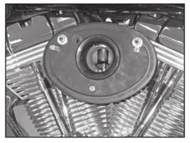
17. Install the back plate and secure with the stock breather bolts. **NOTE: Do not completely tighten at this**
