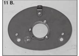
11. Install the three stand-offs onto the backing plate using the three bolts from the previous step.
