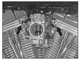
13. Install the breather extensions into the stock breather bolt location as shown.
