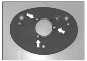
10. Install the three backing plate mounting bolts through the velocity stack as shown.
