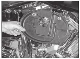
4. Remove the stock air filter base from the engine as shown.
