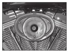
19. Install the K&N air filter and secure with the three bolts provided.
