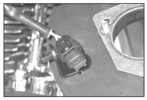
16. On vehicles equipped with an intake valve solenoid, install the intake valve solenoid connector into the bracket installed onto the rear of the backing plate. Secure with the provided tie wrap.
