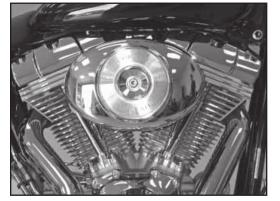
20. Reinstall the factory chrome cover and secure with the factory bolt. **NOTE: Be sure to not over tighten the mounting bolt and distort the cover.**
