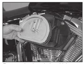
2. Remove the three bolts which secure the stock air filter element. Then remove the stock air filter element and stock crank case breather hoses as shown. NOTE: The stock breather hoses will not be reused with the K&N custom assembly.
