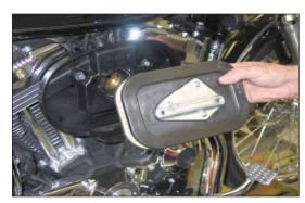
4. Remove the air filter as shown.
