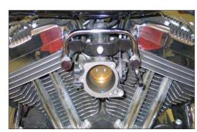
7. Install the K&N crank case breather tube onto the vehicle using the provided hardware.
