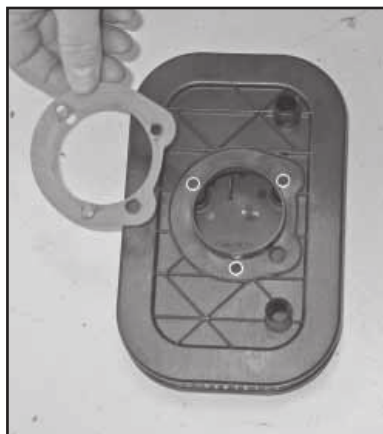
5. Remove the stock air filter gasket from the stock filter.
