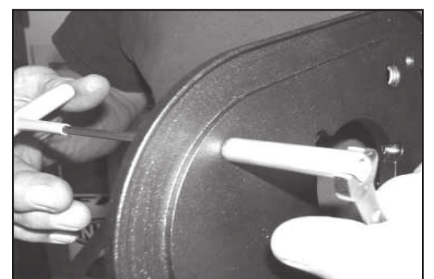
8. Install the four bolts from step 8 through the back plate and thread the bolts into the provided spacers. NOTE: Apply the provided thread locker to four of the provided button socket bolts.
