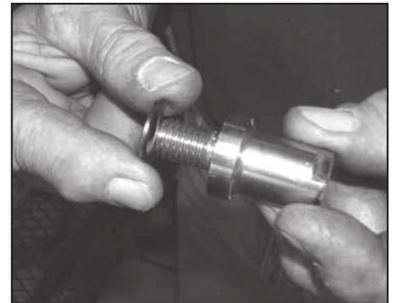
6. On carbureted models, install one of the provided washers onto each of the breather bolt extensions. NOTE: On fuel injected models the washers will not be used.
