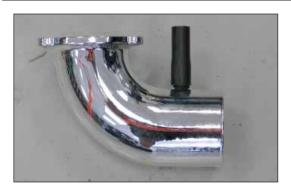
10. Cut the provided crankcase vent hose to a length of 1.75" and install onto the K&N® intake tube as shown.
