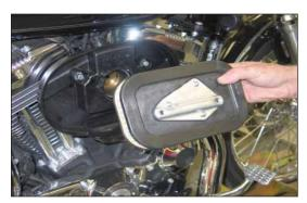
4. Remove the air filter as shown.
