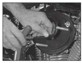
18. Tighten the three bolts that secure the back plate to the throttle body/carburetor. Then tighten the two breather bolts fully.
