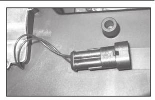
5. Some models are equipped with an intake valve solenoid connector on the back of the stock air filter back plate. Unhook the connector from back plate.
