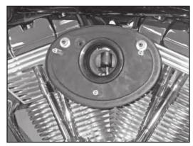
17. Install the back plate and secure with the stock breather bolts.
