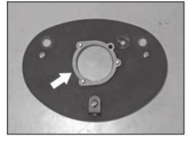
14. Install the provided gasket onto the K&N backing plate as shown.
