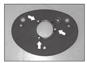
10. Install the three backing plate mounting bolts through the velocity stack as shown. NOTE: Apply the supplied thread locker to the threads of the three supplied stand-off bolts.
