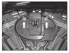
Remove the stock breather bolts which secure the stock air filter base shown.
