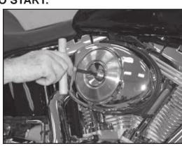
1. Remove air filter cover mounting bolt and cover from the vehicle as shown.
