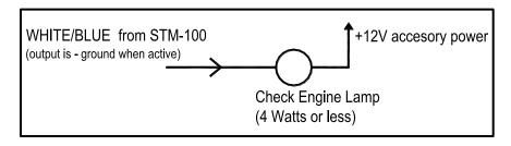
If you need the check engine output to be "active high" or provide a +12V voltage when active a standard 12V relay can be used to accomplish this.
