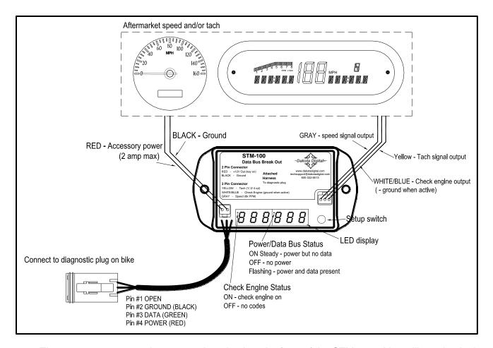
There are two separate harnesses that plug into the front of the STM-100. You will need to look at the instruction for your gauge and connect the STM-100 wires to the appropriate wire.
